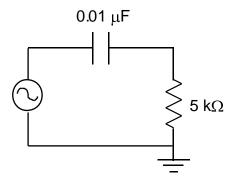
(a) Find the rms current <u>and</u> its phase angle relative to the input signal from the function generator (assume this has zero phase).
