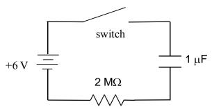
(a) Carefully sketch the <u>voltage across the resistor</u> vs. time. Be sure to label the axes and the scales on the graph. Also, show any calculations you make.
