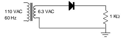
(a) Carefully sketch the voltage across the resistor (as a function of time) for the circuit above. Be sure to label the maximum and minimum values of the voltage. Also, show any calculations.
