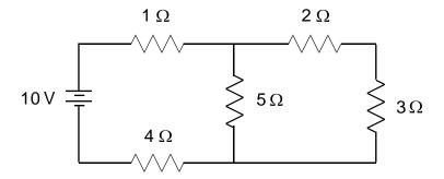
(a) Calculate the current through the 4- $\Omega$  resistor.
