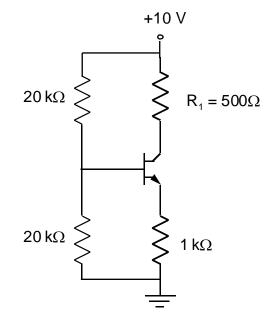
(a) What is the approximate current through the resistor  $R_1$ ?
