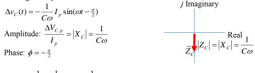
$$\vec{Z}_{c} = j \frac{-1}{C\omega} = \frac{1}{C\omega} e^{-j\frac{\pi}{2}} = \frac{1}{C\omega} \angle -\frac{\pi}{2}$$
