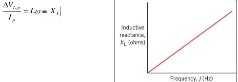
Now we have the inductive reactance  $|X_L| = L\omega$  determining how much voltage is required for a given current.
