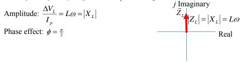
$\vec{Z}_L = jL\omega = L\omega e^{j\frac{\pi}{2}} = L\omega \angle \frac{\pi}{2}$ (the factor of *j* plays the roll of  $\hat{y}$  to indicate the direction is along the Imaginary axis)
