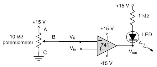
E. Set the reference voltage to about 5 V. Use another 10k pot to input an adjustable DC voltage.
