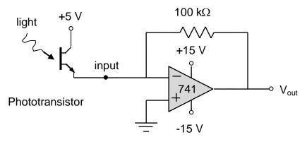
B. Observe what happens to the output voltage with a DMM as the phototransistor is covered and uncovered.
