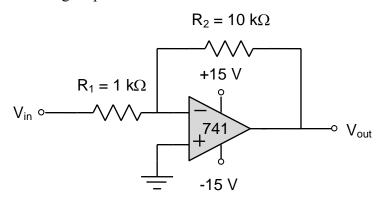
D. Input a sine wave with an amplitude of 1 V and a frequency of about 1 kHz and observe the output.
