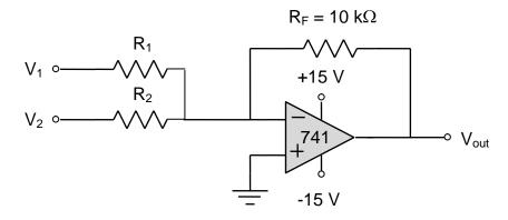
B. Input two different DC voltages for  $V_1$  and  $V_2$  (such that  $|V_1+V_2| < 12V$  or the op-amp will max out) and measure the output.
