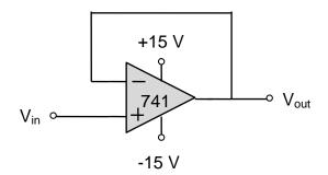
D. Input a sine wave with an amplitude of 5 V and a frequency of about 1 kHz and observe the output.
