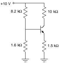
2. For the circuit below, suppose  $\beta = 50$  for the transistor and the input voltage (v<sub>IN</sub>) is +2.5V?
