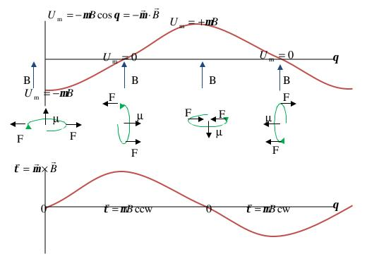
Notice that, while there is no torque on the loop either at its energetic minimum or maximum, *just* off those points there is some. At theta=0, a minimum, if the loop were twisted a little
