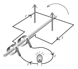
It requires energy to turn the generator because the magnetic force on the loop opposes the motion. A careful calculation shows that the mechanical power input into the generator is the same as the rate energy is transferred to thermal form.
