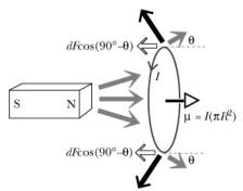
It is difficult to calculate the distance dependence of the force based on the figure above, but we do see that there would not be a net force in a uniform magnetic field.
