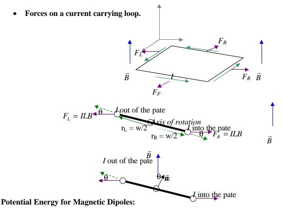
We can phrase the same interaction in the language of work and energy. When the loop rotates a small angle  $d\mathbf{q}$ , the sides of length w move a distance  $(w/2)d\mathbf{q}$  in the direction of the perpendicular part of the magnetic force. Suppose the loop starts at an angle  $\mathbf{q}_i$  and rotates to an angle  $\mathbf{q}_f$ . The magnetic potential energy is the negative of the work done by the magnetic force. There are forces on both sides of the loop, so:
