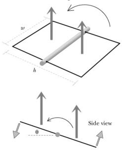
The emf is largest when the angle q is 90°, because the wires are moving the fastest in the direction perpendicular to the magnetic field. The size of the emf on the left wire depends on the component of the velocity perpendicular to the magnetic field:
