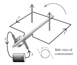
Generators : Suppose a loop rotates at an angular speed w.
