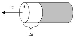
• That means that there are  $N_e = n(A\overline{v}\Delta t)$  electrons passing a point in the wire and the electron current is:
