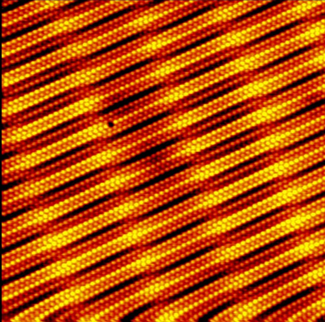
A  $180 \times 190 \text{ \AA}^2$  image of the Pt(001)-hex reconstructed surface taken with a custom Scanning Tunneling Microscope at Aarhus University's Scanning Probe Microscopy lab. The dark spot near the center is a single, missing atom.
