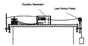
2. Hang 200 grams on the end of the string and start with a very low frequency. Gradually increase the frequency until the amplitude of the wave on the string increases dramatically indicating that you have reached a resonance. You should increase and decrease the frequency to find the value that gives the largest amplitude.
