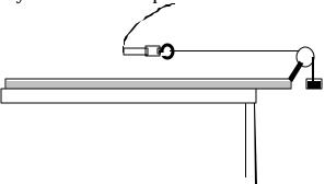
2. Take measurements of the tension in the string for several masses hanging <u>at rest</u> (similar to what you did in Part One) and fill in the table below. The string should be approximately parallel to the track. *Don't forget to Zero the probe first (things shift when it gets tilted horizontal).*
