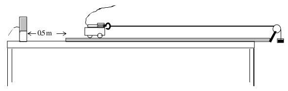
5. Hang about 50 g or 100 g on the string so that the cart moves across the ramp in about 1 to 2 seconds after the mass is released. Record the combined mass of the cart and probe (from Part 2) and the size of the other mass.
