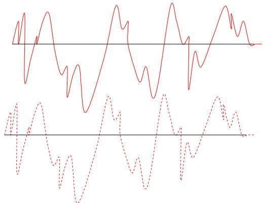
Now, the highest frequency sound that you can hear is around 20 kHz, so to capture undulations with that frequency, you'd need to sample twice as quickly – so you could see a peak, then a trough, then a peak, then a trough,... 40 kHz, or once every 0.0025ms.
