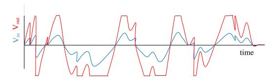
If we're processing sound, clearly, if the amplified & clipped signal drove a speaker, the sound wouldn't just be *louder* than the original, it would be comprised of different high-frequency components (recall that the flat-topped square wave sounds like it's built of lots of higher and higher frequency pure tones)
