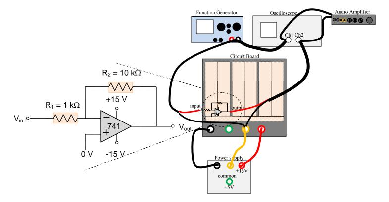
This circuit, with an ideal Operational-Amplifier in it, would simply have a gain of  $-\frac{R_2}{R_1}$ , or, in this case, -10, where the negative sign means that the output isn't just 10 times larger, it's also flipped. Again, since people are relatively insensitive to such changes in phase, we won't worry about that. Unlike with the single transistor, there is no need to offset the input and there is no offset to the output – if the input is a sine wave,
